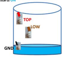
STATUS: when the water in the tank once reaches the top level, the motor will stop. The top and bottom level will start glowing OHT TOP: yellow led GLOW OHT LOW: red led GLOW
