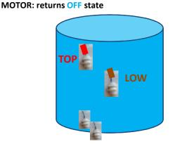
STATUS: Auto cut off if motor Runs dry 120 seconds it shows dry run indication.
